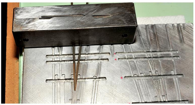
Flow some flux into the joint but be careful not to get it on the outside of the rails or solder will flow out of • the joint. Apply heat and flow enough solder to fill the joint about 3/8-1/2'' or so from end. 18
