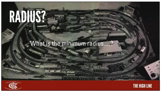
FIGURE 2: While these 80-foot passenger cars may track okay on a 19" radius curve, they look totally toy-like and ridiculous with their extreme overhang and offset. To pick the proper curve radius, this article discusses how to determine a ratio of your rolling stock length that meets your desired performance needs.
