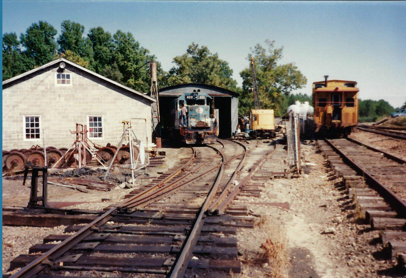
Aberdeen Shops 3-way stub switch, 1992
